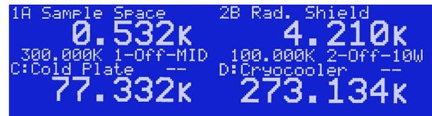
The Home screen projects four user configurable zones that allow the real-time display of all input channel, control loop and instrument status information. From this screen, accessing any of the instrument's configuration menus requires only a single key press.
