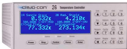
The Model 26 cryogenic temperature controller was designed for applications requiring high output power while still supporting a wide range of temperature sensors. Four inputs and four independent control loops provide a total output power of 150W.
